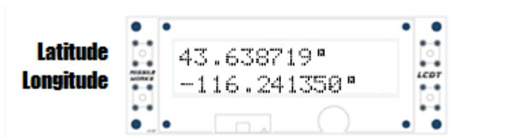
The Latitude coordinate is always shown on top with the Longitude coordinate always shown on the bottom. Coordinates are displayed in the Lat/Lon Format you have selected. This data represents the current or last received coordinates of the ROCKET transmitter.
