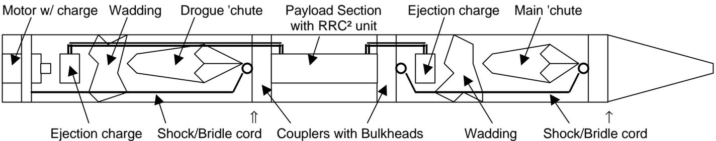
**Two-Stage Recovery System with Forward and Rearward Deployment**
