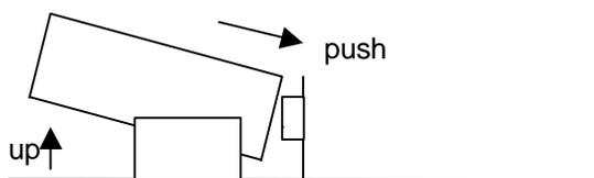
**Figure 4 - Battery end clip placement (side view)**
