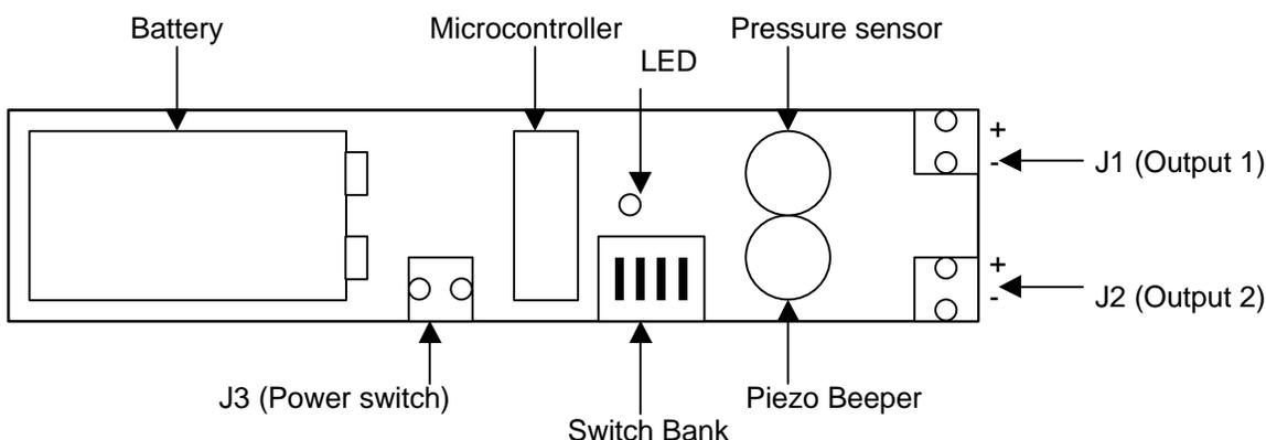
The switches are labeled 1 through 4 accordingly, switch 1 being the leftmost switch as illustrated in figure 1. The ON/OFF position is also labeled, with the ON position being UP, the OFF position being DOWN. The following table describes the switch functions and the corresponding modes of operation:
