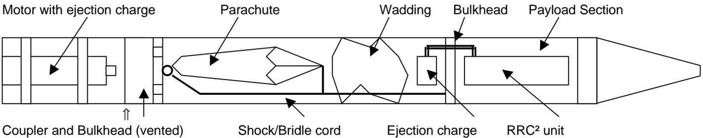
**Two-Stage Recovery System with Forward Deployment**
