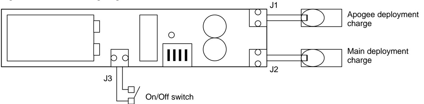
For the most failsafe wiring scheme to minimize the possibility of premature firing of the ejection charges, wire in a pair of normally closed phono jacks or disconnect switches in series with the leads of the deployment charges. The phono jack or switch serves as a disconnect between the unit and the deployment charges.
