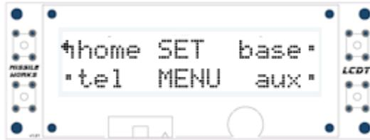
Within the Settings Menu are three sub-menus for three groups of functions: Base (top right button) providing access to the most commonly used functions, Auxiliary (bottom right button) which provides control over the Auxiliary output, and Telemetry (bottom left button) which controls the data stream fed via the on-board com port.
