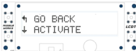
Pressing the top left button will return to the Output Diagnostics menu. Pressing the bottom left button will fire the selected output, then return to the Output Diagnostics Menu.
