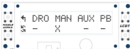
In the example above, there is continuity only on the Main terminals, and the pushbutton is not pressed.
