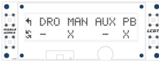
Likewise, connecting a match (or test light) to the Drogue terminals and pressing refresh (while no longer holding the programming push button) results in the following display
