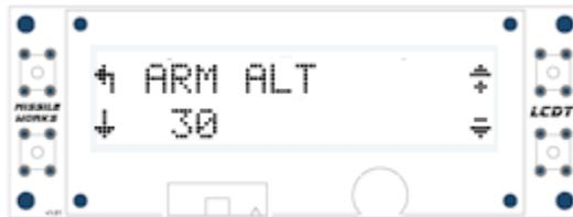
Here, the top left button maintains its function of taking you back one level, and the bottom left button navigates to the next setting. The top right button increases the setting value, in this case the Arm Altitude, until the maximum allowed value is reached, and the bottom right button decreases the value until the minimum allowed value is reached.
