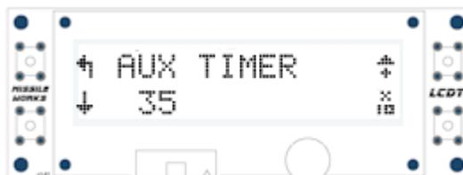
Pressing the top-right button will increment the displayed value by 1. Pressing the bottom-right button will multiply the displayed value by 10. In this case, 35 becomes 350. If the value multiplied by 10 exceeds the permissible range, the value will revert to zero. So, starting with the display above, pressing the bottom-right button once will change the value to 350. Pressing it again will change it to zero.
