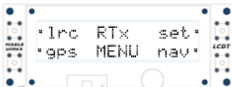
In the RTx Menu, the top left button is used to retrieve the "Last Received Coordinates", the bottom left button invokes a live display of GPS Data (if the optional modules is installed), the top right button brings up the Settings menu, and the bottom right button invokes the "Navigation" screen (using the Last Received Coordinates).
