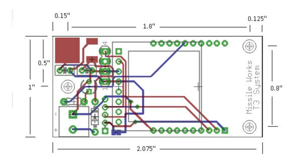
NOTE: All mounting holes are 0.125" diameter (for #4 hardware)
