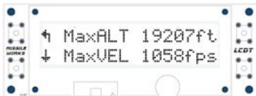
There are a total of 8 pages of data displayed, with the first 5 providing data for the latest flight, and the last 2 providing cumulative statistics for the altimeter. The items displayed, in order of display are:
