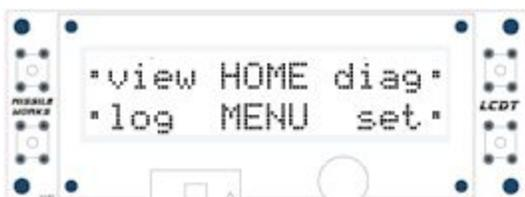
The LCD navigation is based around the four "1-touch" buttons on each side of the display. The center of the display shows the subject/context, and next to each button symbol is an icon or word, describing the button's action.
